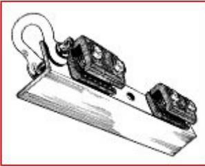
**Frame Rack Jaws with Angle Brackets**
