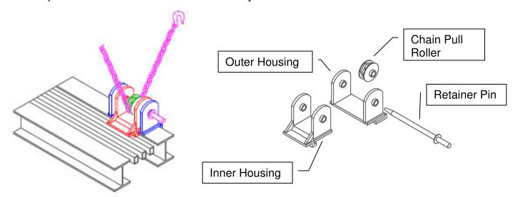
Inner housing and outer housing mate via the retainer pin and attach to the treadway.
