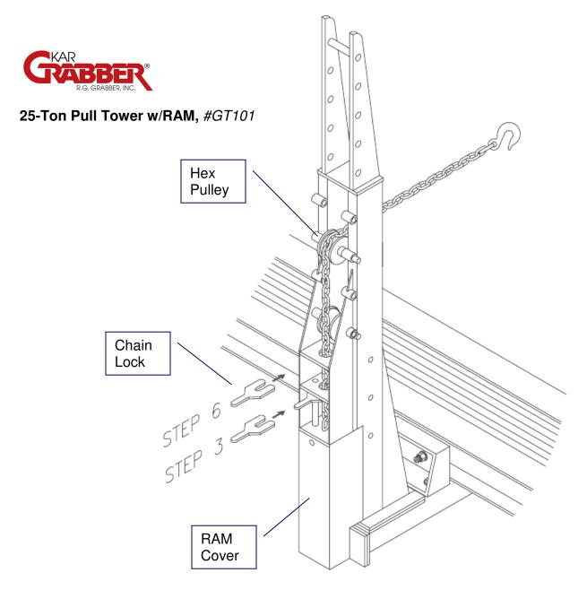
**Step 1.** Thread the pull chain over the top pulley and through the fixed plate and pull plate.
