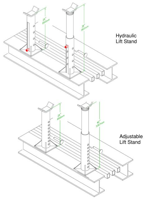
The **adjustable stand** has all the capabilities as the hydraulic stand except that it is adjusts manually. Height range from 6" - 42" at 1-1/2" increments.
